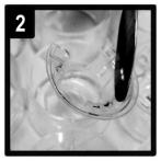
The insert housing keeps constructs from floating during staining; it pins down the construct without affecting macrostructure.
