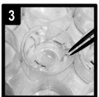
Each VHSE should be totally submerged when staining. For long term storage, allow the construct to sit in the middle of the well with plenty of PBS.
