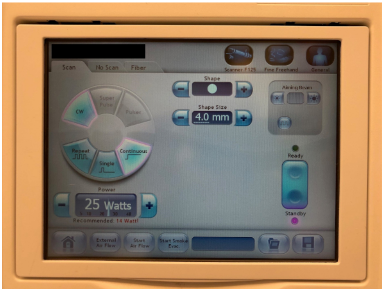
Figure 1: Photo of laser settings. Standard laser settings for CO2LT on the laser system used. Please click here to view a larger version of this figure.
